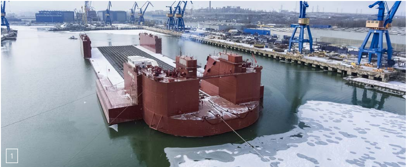
1. The launching barge at Vard Tulcea was enlarged into a fully-fledged floating dock during 2016.
