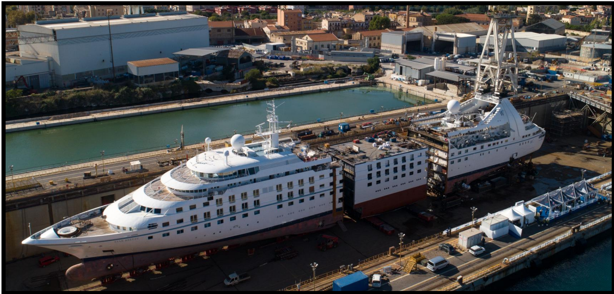
Caption: Windstar Cruises' Star Breeze is cut in two, with the new section inserted, at Fincantieri's Shipyard in Palermo.
