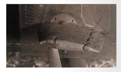
Results of the basic comparison between Fincantieri unflapped and flapped profiles used for type SR retractable fin stabilizers and NACA coded profile, following cavitation tunnel tests.
