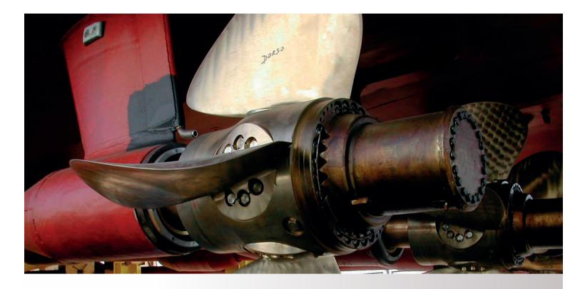
— The additional technical advantages related to the feathering configuration cannot be omitted: the maintenance and operating cost reductions following the capability to operate with one propulsion line and the other in "flag position" instead of both shaftlines at low rpm are quite remarkable both in terms of fuel consumption and operation at design pitch and following improved margin against cavitation.
