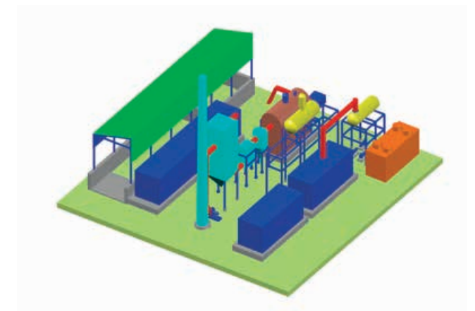
— 200 kW Biomass Plant
